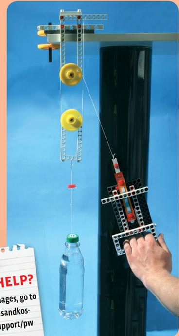
But you can achieve an even greater savings in force. The more pulleys the combination pulley has — more accurately, the more strings there are running to and fro — the more force you save. The load is simply divided by the number of strings.
