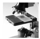
5) Next, choose the magnifying power you want to use. Your microscope can provide magnifying powers of 50X, 100X, 150X, 300X, and 600X. Remember that the longer objective lenses used with the higher magnification 20X eyepiece provide the higher powers. For optimal viewing, start at the lowest power and work your way upward. Most observing is done at low power.
